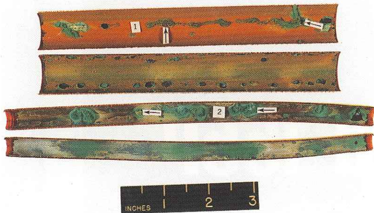
PHOTO A. Soldering-flux-induced pits covered with friable green tubercles of copper-corrosion products. The tube-wall perforations (see arrows) and most of the pits exist along relatively narrow bands, which are nearly parallel to the longitudinal axes of the tubes (i.e., along the “ghosts” of flux runs).
