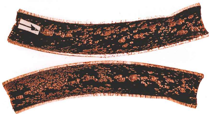
PHOTO D. A tube-wall perforation (see arrow) in a localized area of severe cavitation. Surface heating caused the formation of black cupric oxide where cavitation had not occurred.
